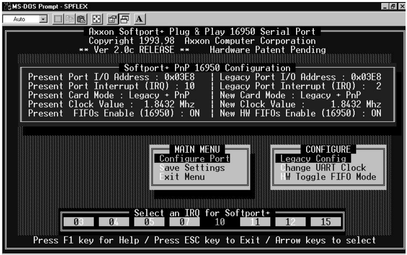
SpFlex Legacy IRQ Configuration for Axxon ISA 16x50 with Flex-Clock Product in Non-Plug & Play Environments
